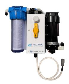
**Dual Prefilter Filter Bowls** Locate in an area that allows easy access as these will be the most frequently serviced module while cruising. Mount vertically and leave room below bowls for filter changes. Do not mount above water-sensitive equipment.
