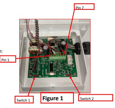
Auxiliary Outputs 1 and 2 are switched to the supply voltage when turned on. These outputs are protected by 100mA self resetting fuses.
