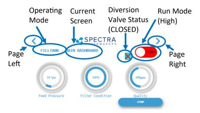
6. When the Product Water Quality is below the programmed threshold, the Diversion Valve opens, allowing water to enter the tanks and the screen image changes.
