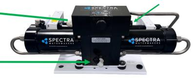
Spectra Clark Pump and Pressure Vessel/Membrane: Mount in a cool location (below 120 deg. F/49 deg. C). May be oriented in any position and can be well above waterline. Leave access to the pressure relief valve. Do not mount over electrical equipment. Use supplied spacers and washers for the vibration mounts.
