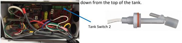
The float switch must be connected to the Tank Switch 2 terminals on the Spectra Connect control board at the Feed Pump Module. There is no polarity.
