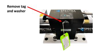
Open the pressure relief valve On Clark Pump:
