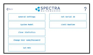
**System Model:** Configures the Spectra Connect for a different system model from a preset list of options. **Clear Statistics:** Resets all of the Estimated Maintenance Intervals back to 100%. This feature should only be used on a brand new system.
