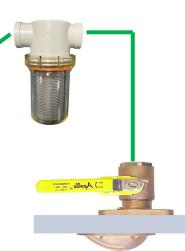
1/2" or 3/4 scoop strainer thru-hull and Seacock: Mount low, in a clear flow and away from head discharge.
