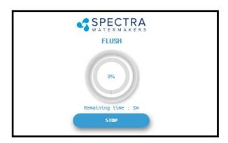
8. After Fresh Water Flushing the system will enter the 'Auto Store' mode, and the interval timer until the next scheduled flush will show on the screen.
