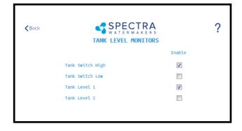
**Tank Setup** - Enable/disable tank sensors.
